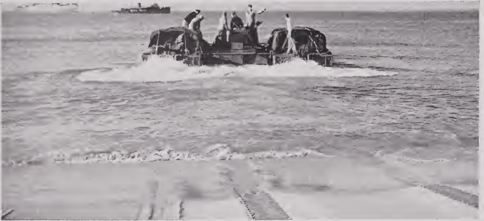
FIGURE 64. Wet ferry test: medium tank supported by two DUKWs leaving beach at Fort Story.
